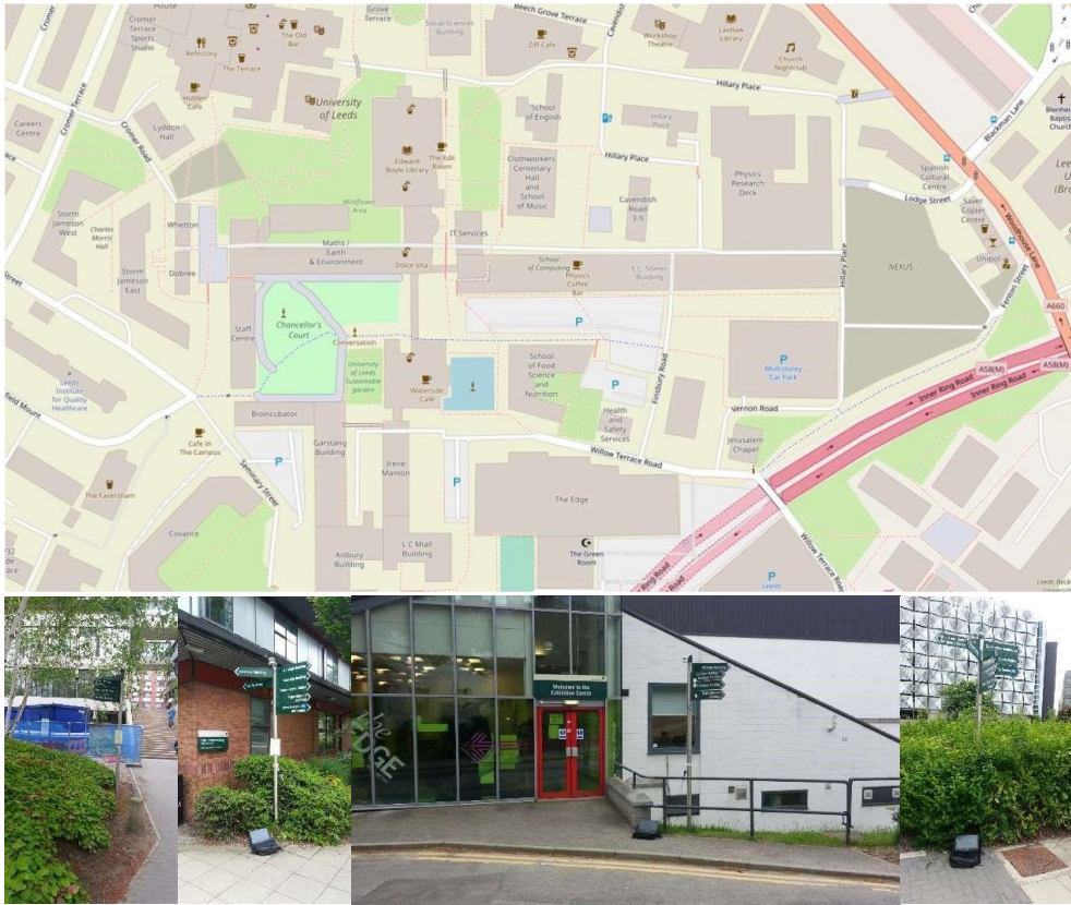
Figure 2. Precinct surrounding Waterview Café (upper pane), with four radiation-screened temperature sensors deployed to monitor micro-climate variations (lower panes). In the map please find Chancellor's Court (light green); the Cooling Pond (blue); Cark Park south of the EC Stoner Building (grey); and the Edge on Willow Terrace Road
